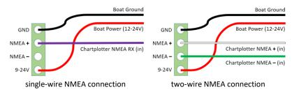
By default, dAISy 2+ is configured to output at 38400 Baud (NMEA high speed). This can be changed to other baud rates in the configuration and debug menu. You also need to check the configuration of your chartplotter. In many models, the NMEA port needs to be enabled in the settings menu and set to the correct protocol, like for example NMEA high speed).
